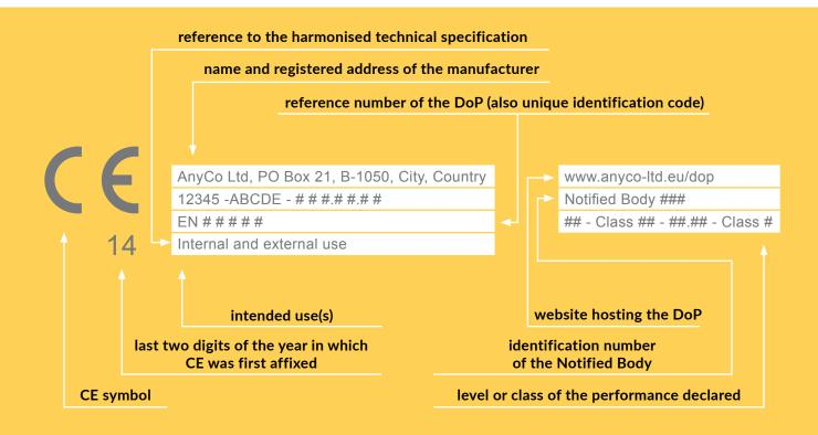
EXAMPLE: Bulk aggregates are usually CE marked in the accompanying documents, usually together with the despatch note provided by the manufacturer.
